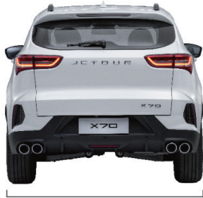
Wheel tread: 1,900 Wheel tread : 15 (front/rear) - 1,563/1,577
